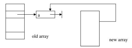
Addition of variable: A new node is added to the head of the new array, chained to the old variable node. [2]
